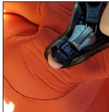
Figure 1: Bottom of zipper failure due to glue separation.
